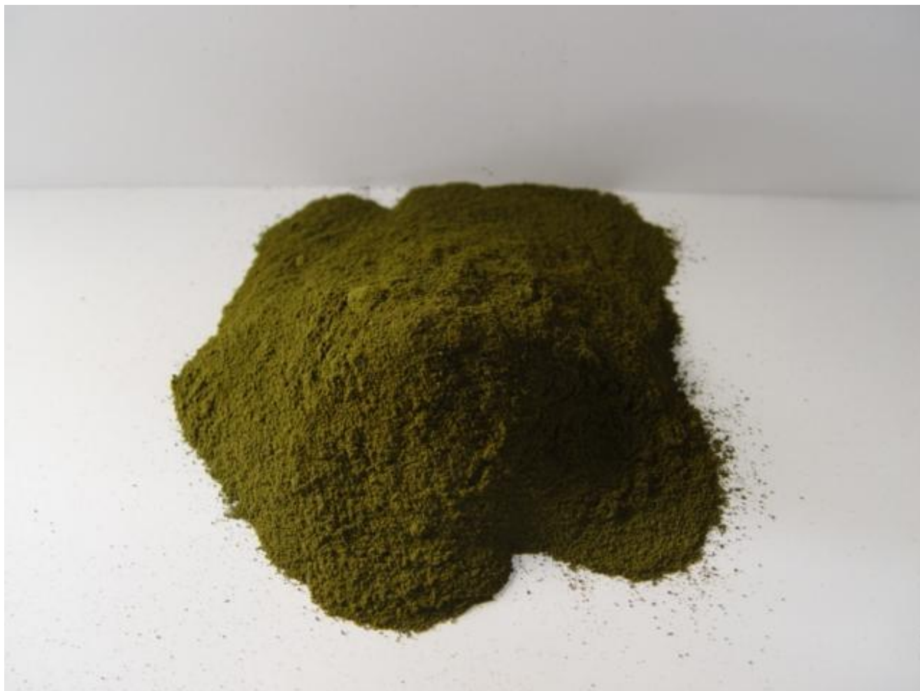
Picture 6. A photograph of the pulverized Dunaliella tertiolecta algae post mill grinding..
