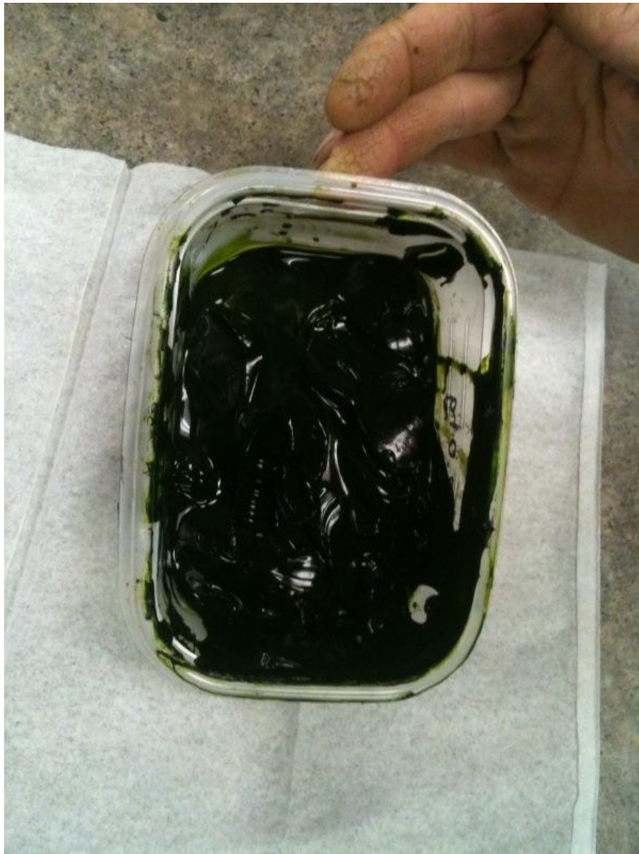
Picture 4. Dunaliella tertiolecta algae paste post harvesting with the centrifuge (not dried yet).
