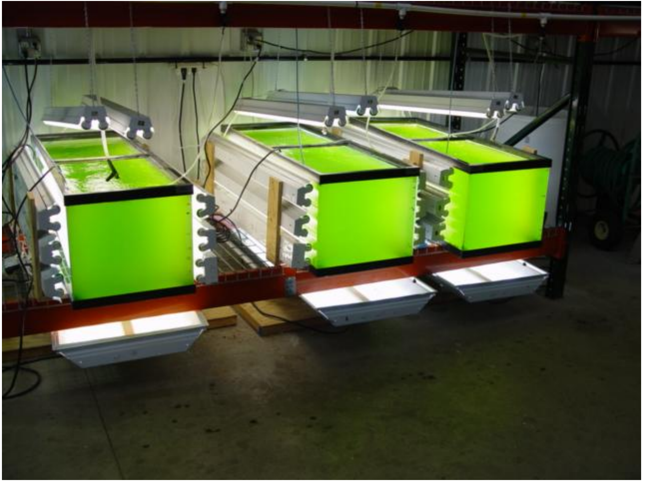
Picture 2. A photograph of Dunaliella tertiolecta algae grown with artificial light inside (aquariums).
