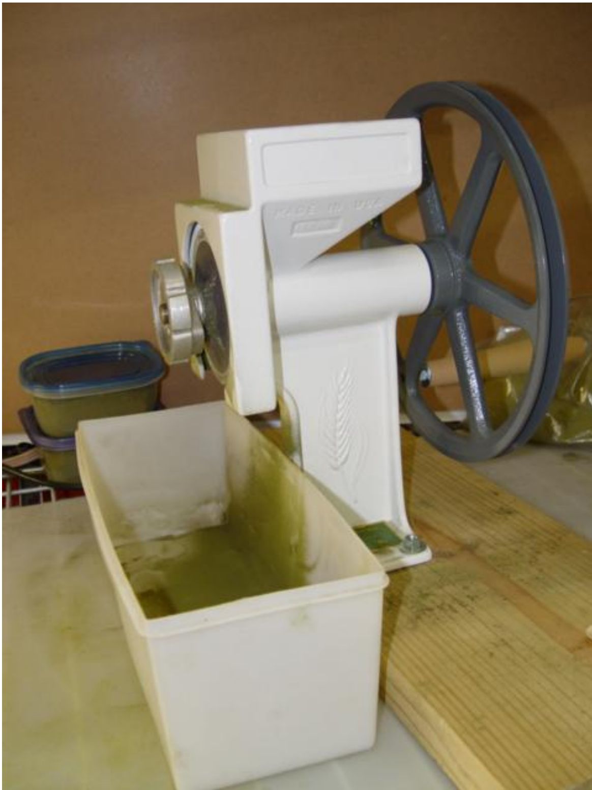
Picture 5. A photograph of the mill used for pulverizing the dried Dunaliella tertiolecta algae.
